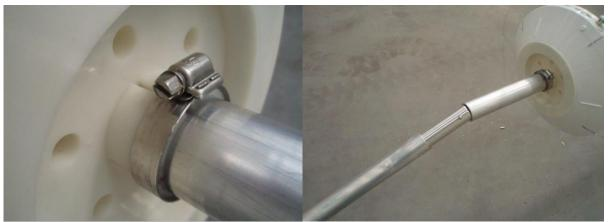
Mount the extension axis on the turn axis for 6 row operation.
