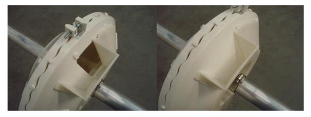
Make sure that the 4 drums have the same adjustment of the amount of material coming out of the drum.
