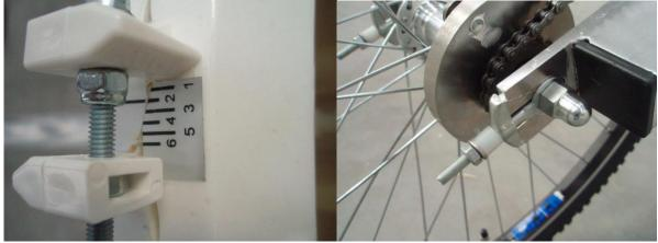
Adjustment of the chain gear
