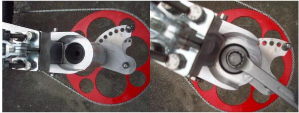
Mount the drums on the axis and fasten the clip with the screwdriver.
